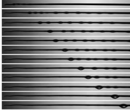
FIGURE 19. Successive snapshots (interval between each picture: 5 s) showing the evolution of a liquid film (thickness 8–25 \mu\text{m} ) made of silicone oil ( \eta = 20 \text{ mPa s} and \gamma = 20 \text{ mN m}^{-1} ) deposited on a conical fibre (of radius between 100 and 300 \mu\text{m} ).
